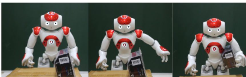
Figure 14. Left Hand- Torso Grasp away from the robot. The on-board SONAR sensor of NAO has a detection range of 20 – 80cm from the robot. Hence the object was always in the SONAR dead-zone. Thus, the sensor data could not be used to automate the proposed algorithm as it was unreliable for determining the position of the object.
